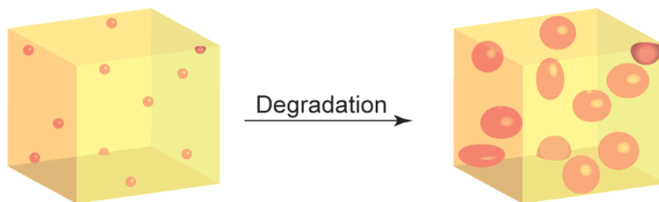
Figure 6. Model for heterogeneous degradation in polymandelide. The yellow volumes are regions where chain scission results in autocatalytic hydrolysis.
